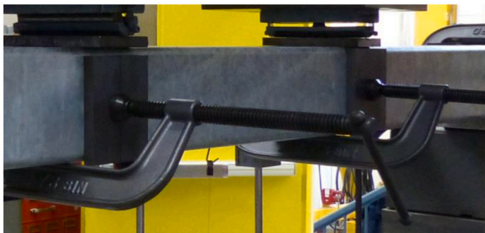
Fig. 3. Reinforcement at load application points and supports.
