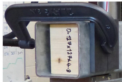
Fig. 3. Reinforcement at load application points and supports.
